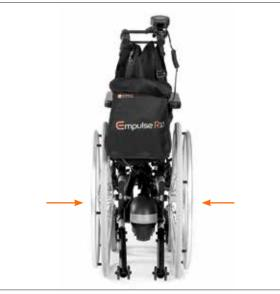
Easy & Convenient Folding The R10 can remain in place when folded.
