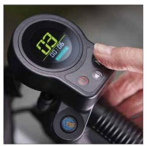
Simple Control Thumb throttle and three push-button speed settings.
