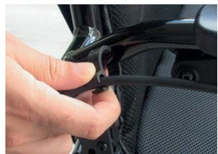
7. To remove battery (which is located under the seat) place your thumb over the back of the battery handle and fingers underneath until clip is located (or alternatively use two hands) , simply press / clench your fingers to pull the clip and simultaneously pull the battery to release it.
