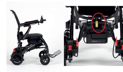
4. Put freewheel levers into ‘Electric’ mode by pushing forward both levers towards the chair. Press in the latch and extend the anti-tip wheel backwards, on both sides of the powerchair.
