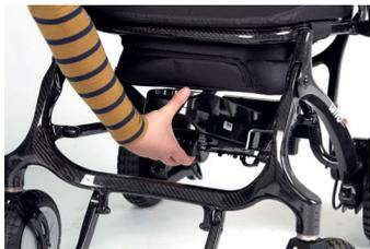
8. To insert battery. Slide the battery on to the rails underneath the seat. Push the battery firmly backwards until it locks in position with an audible click.
