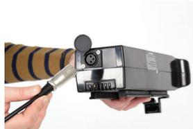
12. Ensure the charger is removed before operation and switch the powerchair on using the joystick.
