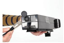
The LED on the charger will appear blue while charging. When charging is complete, the LED will change to green. It is recommended to charge for 5-8 hours on each charge. After charging is complete, remove the charger from the powerchair/battery and the plug from the wall socket. Store the charger in a safe location.
