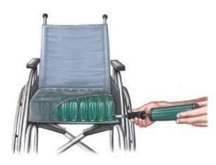
Inflate the CONFORM® Air Cushion with the enclosed pump until it begins to arch. Attach the pump tubing to the cushion valve. Open the valve by turning it anticlockwise and inflate the cushion. Close the valve by turning it clockwise.
