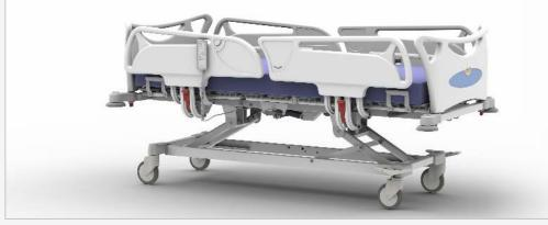
ELECTRIC HEIGHT ADJUSTABLE Height adjustable system by articulated trapezes electrically operated by 2 linear motors Linak brand. Lifting stroke of 380 mm and a maximum patient load of 250kg.
